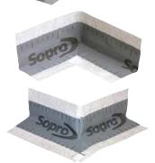
System-tested, highly elastic, nonwoven-backed sealing tape for flexible, trouble-free waterproofing of perimeter and movement joints, and elastic fittings for durable sealing at internal and external angles, for use in conjunction with liquid-applied Sopro waterproof membranes below ceramic coverings.
