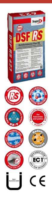
Reactive, sag-resistant, one-component mineral sealing slurry for production of flexible, crack-bridging waterproof membranes. For waterproofing indoor spaces to DIN 18534, for waterproofing tanks and pools to DIN 18535, for waterproofing normal, recessed and access balconies to DIN 18531 Part 5, and for waterproofing elements in contact with soil to DIN 18533. For fixing and bonding
